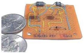
The chip on the left is the iPic microcomputer, based on a PIC 12C509A, in a tiny 8-pin SO8 package. The chip to its right is a 24LC256 EEPROM chip -- it holds all the files that the iPic web-server serves out -- this is roughly like the hard disk on a regular sized computer. The tiny component at the bottom serves as the power-supply regulator
